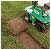
A sod cutter is a piece of gardening equipment that separates sod or grass from the soil. It is a viable alternative to manually removing sections of sod from the ground with a shovel or hoe, which can be messy and time-consuming and can strain the back. Use a mechanized sod cutter for larger areas. A sod cutter is especially useful if your existing lawn is alive and thick.
